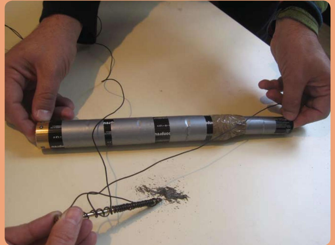
Figure 3: Several batteries connected to an electrical wire to show the movement of the iron chips when current flows.
