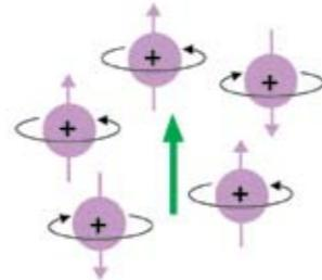
Figure 6: A magnet. Dipoles are oriented in a particular direction, resulting in a global magnetic field.
