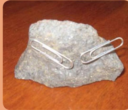
*Figure 8: Clips attracted by a piece of magnetite*
