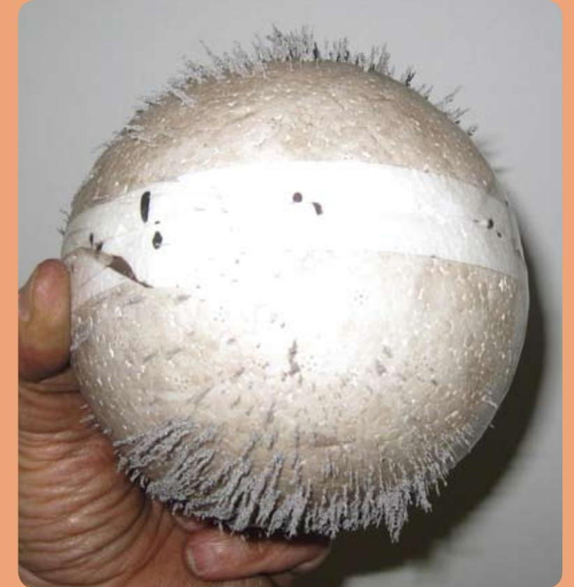
Figure 15 and 16: The iron filings around the magnetized Earth indicate the direction of the poles. As they collect many more filings in this area compared to the equator we can deduce that the magnetic field is stronger at the poles than at the equator.
