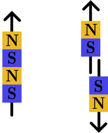
Figure 10: The direction of the two magnetic fields coincides when we bring the north pole close to the south pole, but when we bring together the two south poles, they repel because the two directions of the field are opposite.
