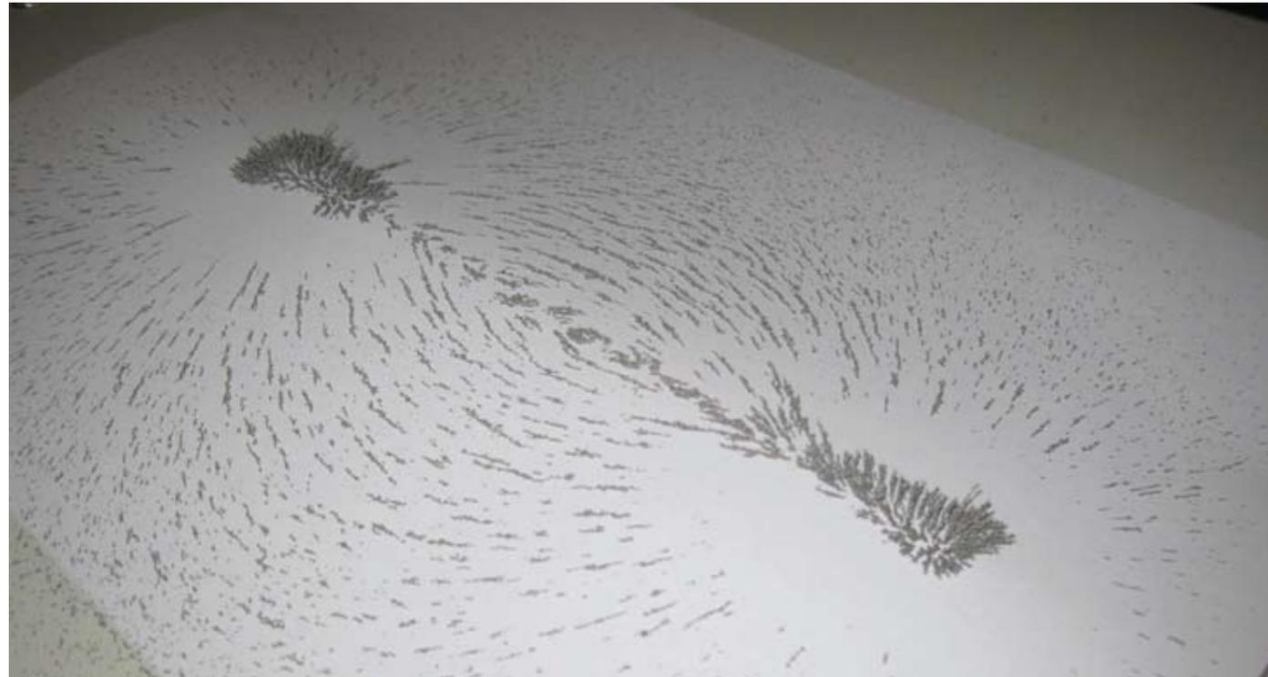
north pole and go into the south pole (figure 12). This means that if we spread iron filings around a magnet they will line up along lines that are similar to those in the Figure. Through the magnetic field lines we can determine where exactly the magnetic force is stronger. Indeed, it can be very intense, as happens in the poles, where the field lines are very dense, or very weak in the middle, where the field lines are far apart.
