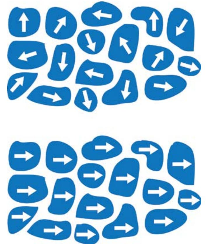
Figure 7: Top, disoriented dipoles, bottom oriented dipoles.
